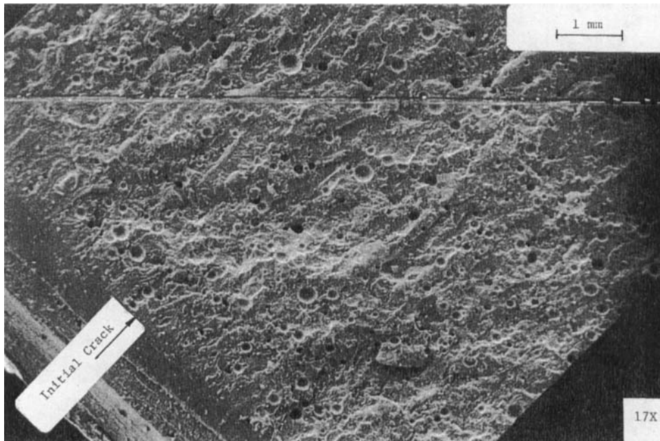
FIGURE 10 SEM fractograph of a Metlbond 1113-2 specimen showing the initial crack, the slow growth whitened and the fast growth regions (1000-min cure at 93°C and fast-cooled); whitened zone ~1.27 mm.
